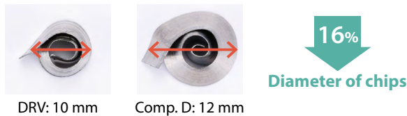
Chip shape comparison of outer insert cutting edge (In-house evaluation)
